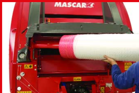
Montaggio bobina rete Installation net reel Montage bobine filet Montage rollo malla
